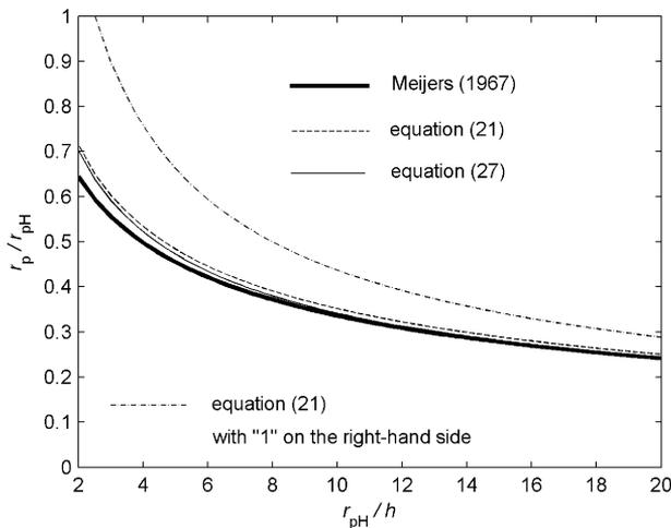
Fig.2: Variation of  $r_p / r_{pH}$  with  $r_{pH} / h$  for a cylindrical indenter;  $r_{pH}$  is the Hertzian contact width
