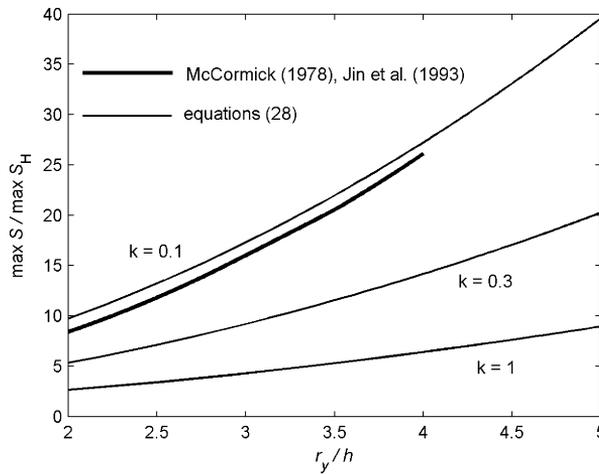
Fig.4: Variation of  $\max S / \max S_H$  with  $r_y/h$  for an ellipsoidal indenter with  $k = R_y/R_x = 0.1, 0.3$  and  $1$ ;  $\max S_H$  is the maximum Hertzian contact pressure for the spherical indenter with radius  $R_x$
