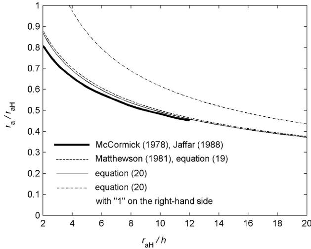
Fig.3: Variation of  $r_a/r_{aH}$  with  $r_{aH}/h$  for a spherical indenter;  $r_{aH}$  is the Hertzian contact radius
