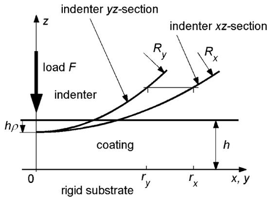
Fig.1: Indentation of an elastic isotropic incompressible coating by a rigid frictionless ellipsoidal surface (elliptical paraboloid)
