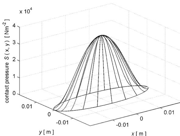
Fig. 5: The contact pressure distribution  $S(x, y)$  for an ellipsoidal indenter with  $\mu = 0.3$  MPa,  $h = 2$  mm,  $R_y = 0.5$  m,  $k = R_y/R_x = 0.1$  and  $F = 10$  N
