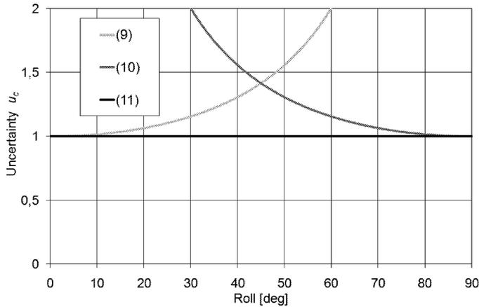
Fig.5: Graphical illustration of the uncertainties of determining the roll
