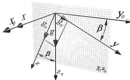
Fig.3: The roll angle against the components of the gravitational acceleration
