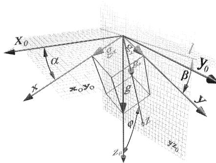
Fig.2: The tilt angles and distribution of the gravitational acceleration
