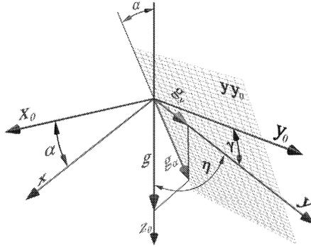
Fig.6: The component of the gravity vector against angles  $\alpha$  and  $\gamma$
