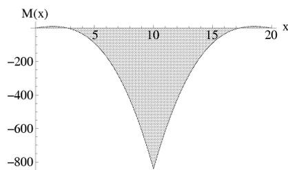
Fig.3: Beam's bending moment, kNm
