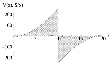
Fig.4: Beam's shear force and shear force at soil bed, kN
