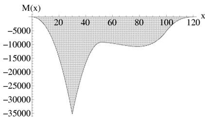
Fig.6: Beam’s bending moments, kNm
