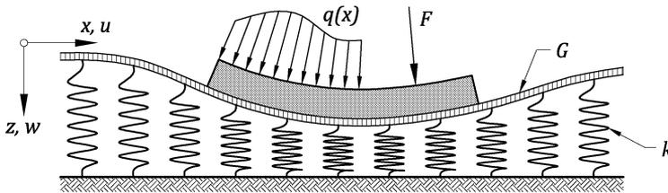
Fig.1: Beam on two-parameter elastic foundation
