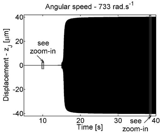
Fig.8: Time history of the centre of the rotor journal displacement in the z-direction ( $k_p = 5$ ,  $k_d = 1$  s,  $\omega = 733$  rad s<sup>-1</sup>,  $e_T = 16.5$   $\mu$ m)
