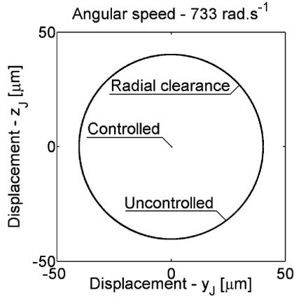
Fig.7: Orbits of the uncontrolled rotor and the rotor controlled by a PD controller ( $k_p = 5$ ,  $k_d = 1$  s,  $\omega = 733$  rad s<sup>-1</sup>,  $e_T = 16.5$   $\mu$ m)
