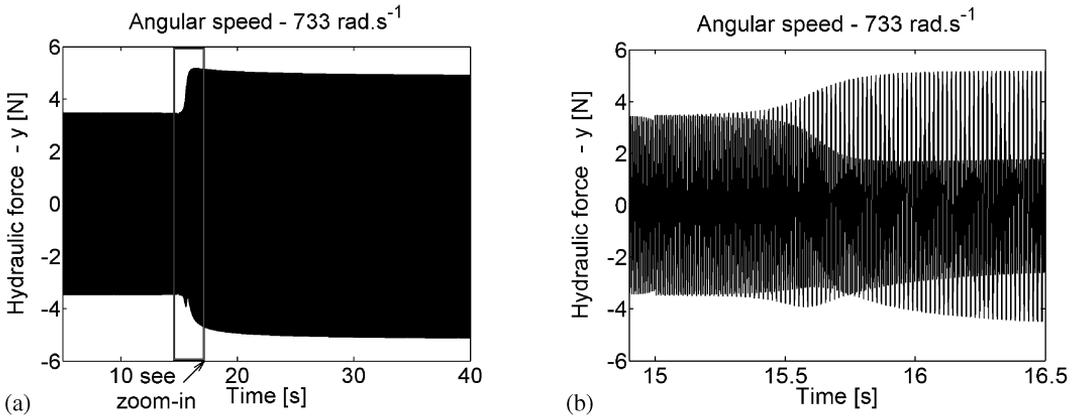
Fig.13: Time history of the  $y$ -component of the hydraulic force (a) and its detail at time 15.7 s (b) ( $k_p = 5$ ,  $k_d = 1$  s,  $\omega = 733$  rad s $^{-1}$ ,  $e_T = 16.5$   $\mu$ m)
