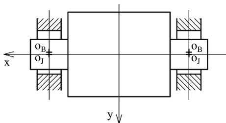
Fig.1: Scheme of the rigid rotor system supported by fluid-film bearings
