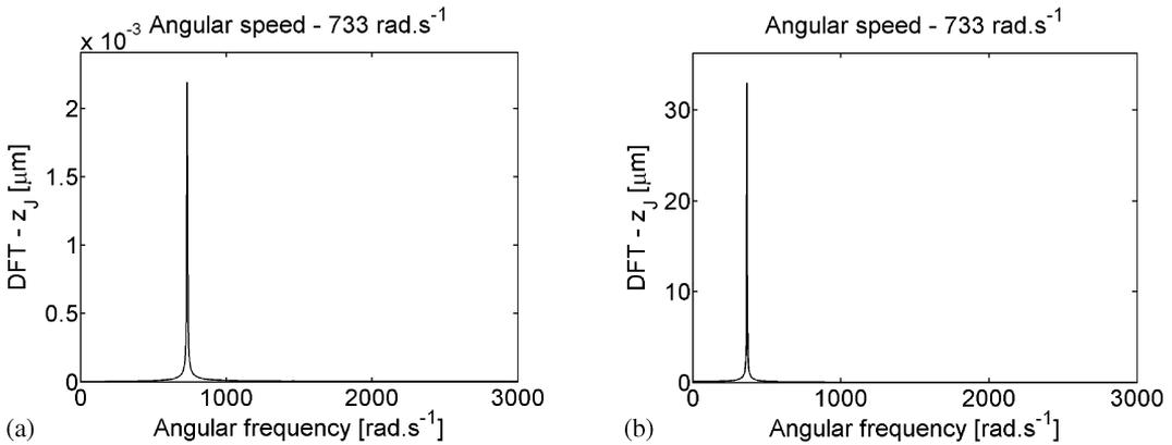
Fig.10: The frequency spectrum of the displacement in the  $z$ -direction of the journal centre of the rotor with a PD controller switched on (a) and off (b) ( $k_p = 5$ ,  $k_d = 1$  s,  $\omega = 733$  rad s $^{-1}$ ,  $e_T = 16.5$   $\mu$ m)
