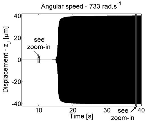
Fig.8: Time history of the centre of the rotor journal displacement in the z-direction ( $k_p = 5$ ,  $k_d = 1$  s,  $\omega = 733$  rad s<sup>-1</sup>,  $e_T = 16.5$  μm)
