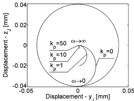
Fig.4: The equilibrium position of the uncontrolled rotor and of the rotor controlled by the P controller
