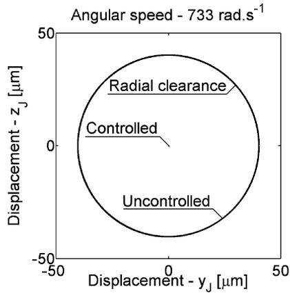
Fig.7: Orbits of the uncontrolled rotor and the rotor controlled by a PD controller ( $k_p = 5$ ,  $k_d = 1$  s,  $\omega = 733$  rad s<sup>-1</sup>,  $e_T = 16.5$  μm)
