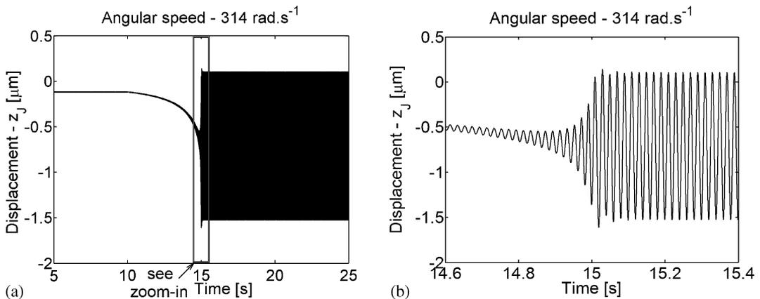
Fig.6: Time history of the centre of the rotor journal displacement in the z-direction (a) and its detail at time 15 s (b) ( $k_p = 5$ ,  $k_d = 1 \text{ s}$ ,  $\omega = 314 \text{ rad s}^{-1}$ ,  $e_T = 16.5 \mu\text{m}$ )
