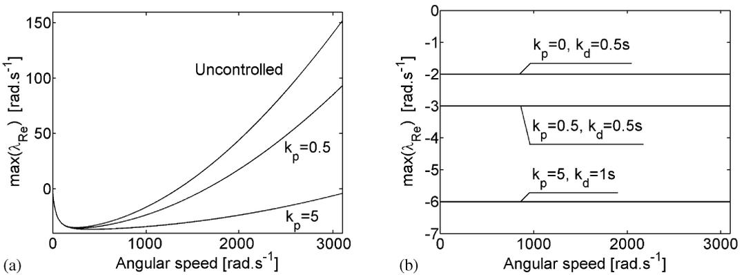
Fig.16: The largest real part  $\lambda_{Re}$  of the eigenvalues of the rotor system with the P (a) and PD (b) feedback controller
