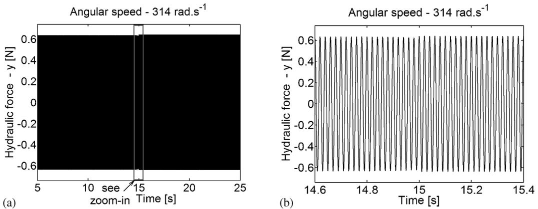
Fig.11: Time history of the  $y$ -component of the hydraulic force (a) and its detail at time 15 s (b) ( $k_p = 5$ ,  $k_d = 1$  s,  $\omega = 314$  rad s $^{-1}$ ,  $e_T = 16.5$   $\mu$ m)
