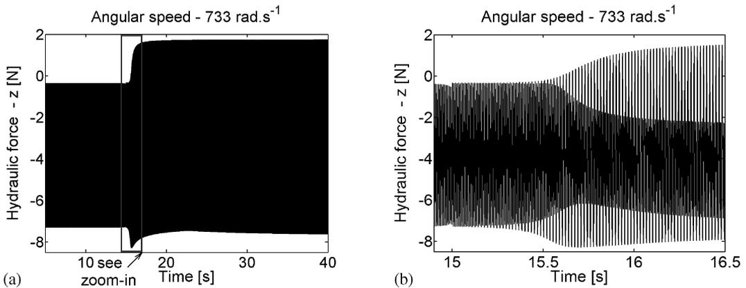
Fig.14: Time history of the  $z$ -component of the hydraulic force (a) and its detail at time 15.7 s (b) ( $k_p = 5$ ,  $k_d = 1$  s,  $\omega = 733$  rad s $^{-1}$ ,  $e_T = 16.5$   $\mu$ m)
