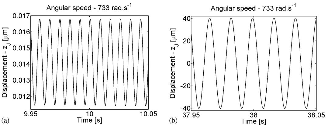
Fig.9: Detail of the time history of the centre of the rotor journal displacement in the z-direction at time 10s (a) and 38s (b) ( $k_p = 5$ ,  $k_d = 1$  s,  $\omega = 733$  rad s<sup>-1</sup>,  $e_T = 16.5$  μm)
