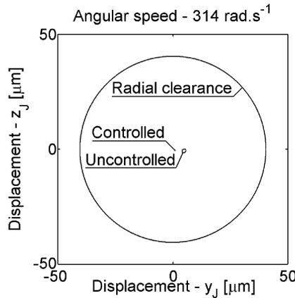
Fig.5: Orbits of the uncontrolled rotor and the rotor controlled by a PD controller ( $k_p = 5$ ,  $k_d = 1 \text{ s}$ ,  $\omega = 314 \text{ rad s}^{-1}$ ,  $e_T = 16.5 \mu\text{m}$ )
