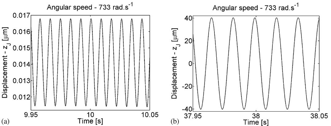
Fig.9: Detail of the time history of the centre of the rotor journal displacement in the z-direction at time 10s (a) and 38s (b) ( $k_p = 5$ ,  $k_d = 1$  s,  $\omega = 733$  rad s<sup>-1</sup>,  $e_T = 16.5$   $\mu$ m)
