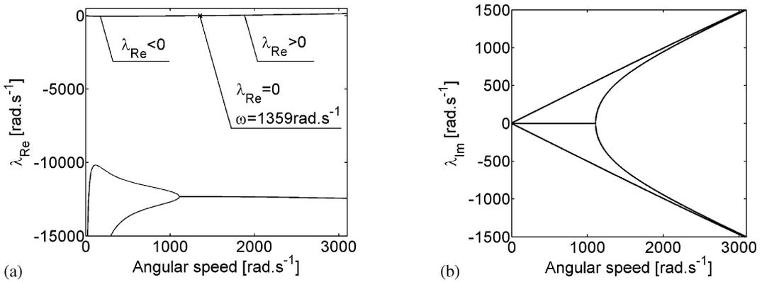
Fig.15: Real  $\lambda_{Re}$  (a) and imaginary  $\lambda_{Im}$  (b) parts of the eigenvalues of the uncontrolled rotor system
