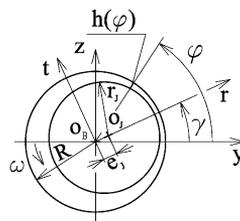
Fig.3: Scheme of a journal bearing
