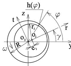
Fig.3: Scheme of a journal bearing
