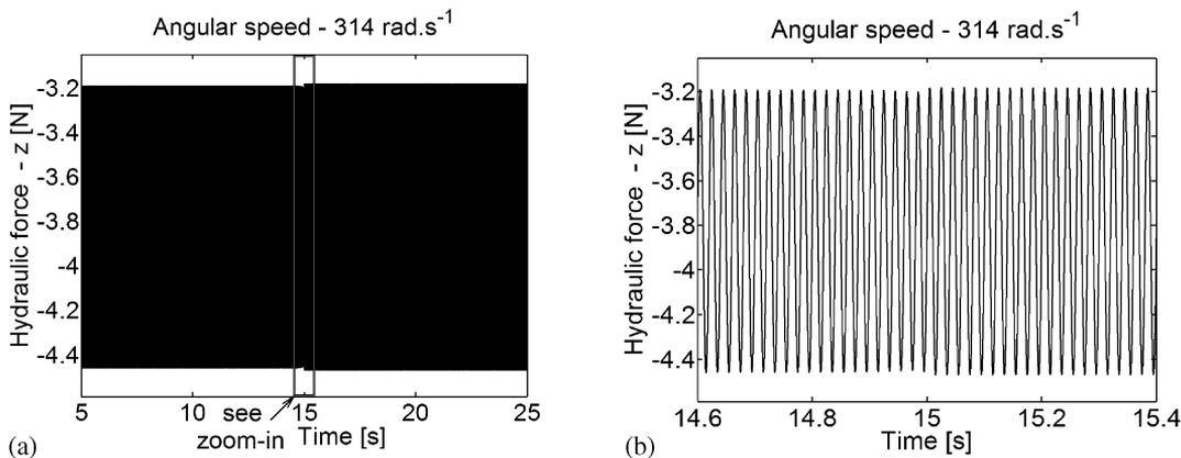
Fig.12: Time history of the  $z$ -component of the hydraulic force (a) and its detail at time 15 s (b) ( $k_p = 5$ ,  $k_d = 1$  s,  $\omega = 314$  rad s $^{-1}$ ,  $e_T = 16.5$   $\mu$ m)
