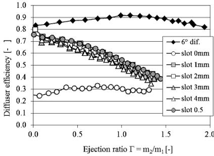
Fig. 7: Diffuser efficiency for backpressure measured at the exit of the diffuser
