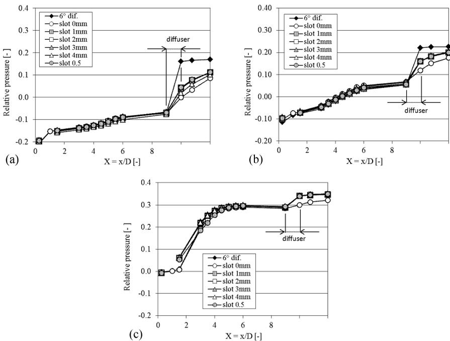
Fig.11: Static pressure distribution on the mixing chamber wall, diffuser and tube after the diffuser for three values of mixing pressure; relative pressure is defined as  $(p - p_{02}) / (p_{01} - p_{02})$ ;  $X = x/D$  is a dimensionless axial coordinate
