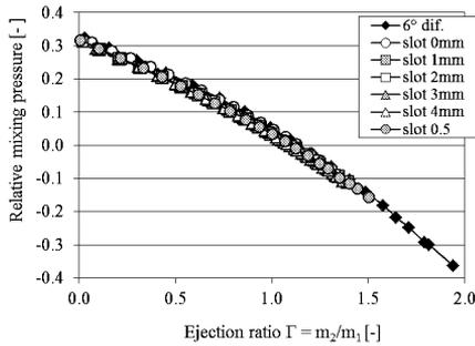
Fig.5: Relative mixing pressure  $(p_3 - p_{02}) / (p_{01} - p_{02})$  at the end of the mixing chamber for various settings of the suction slot
