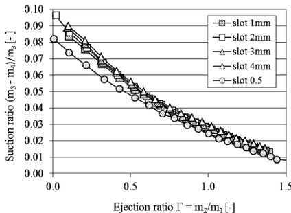
Fig. 9: Suction ratio for various settings of the suction slot and ejection ratio
