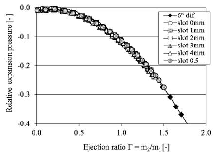
Fig.4: Relative expansion pressure  $(p_{12} - p_{02}) / (p_{01} - p_{02})$  in the beginning of the mixing chamber for various settings of suction
