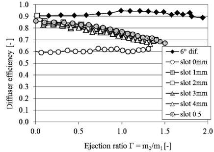
Fig. 8: Diffuser efficiency for backpressure measured 300 mm past the diffuser
