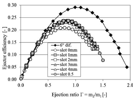
Fig.3: Ejector efficiency for different settings of the suction slot and a comparison with ejector with  $6^\circ$  diffuser [6]
