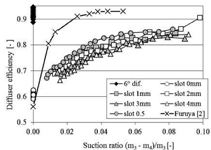
Fig. 10: Diffuser efficiency as a function of suction ratio and slot width
