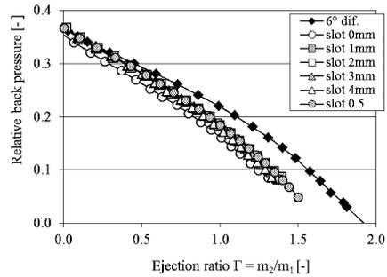
Fig.6: Relative back pressure  $(p_4 - p_{02}) / (p_{01} - p_{02})$  after the diffuser for various settings of the suction slot
