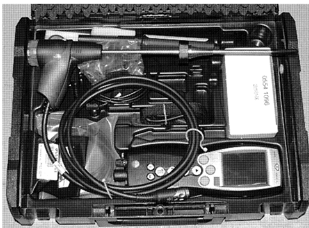
Fig.2: Analyser of combustion gases Testo 330-2 LL
