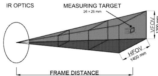
Fig.8: The determination of paper target size
