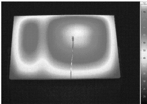
Fig.2: Thermogram of the infrared heating panel – the defective electrical spiral
