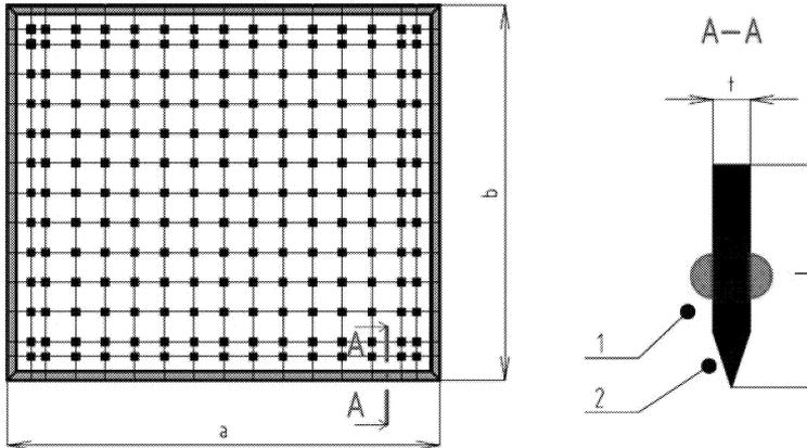
Fig.6: The measuring frame with frame sectional view
