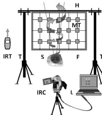
Fig.9: The stand for measuring temperature fields in 3D airflows by the fan with a rotate circle airstream by an infrared camera; IRC – Infrared Camera, L – Laptop, MT – Measuring Targets, T – Tripod, H - Holder, IRT – Infrared Thermometer, S – Source of 3D Non-Isothermal Airstream, F – Frame
