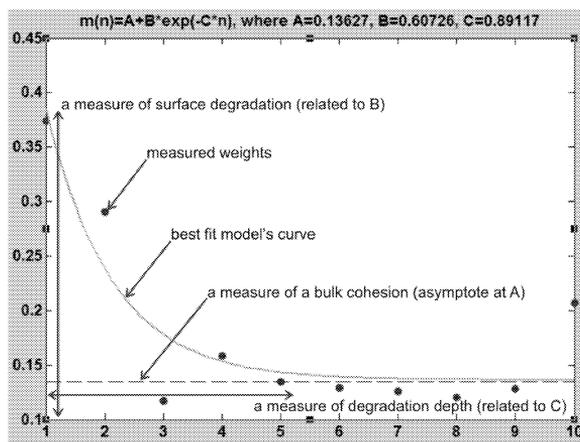
Fig.3: Typical evaluation diagram of peeling test
