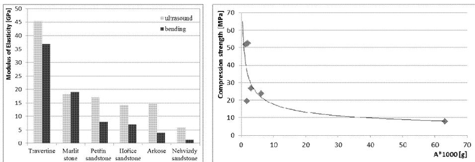
Fig. 7: a) Comparison of MoE obtained from bending tests and ultrasound tests, b) comparison of peeling tests and compression tests
