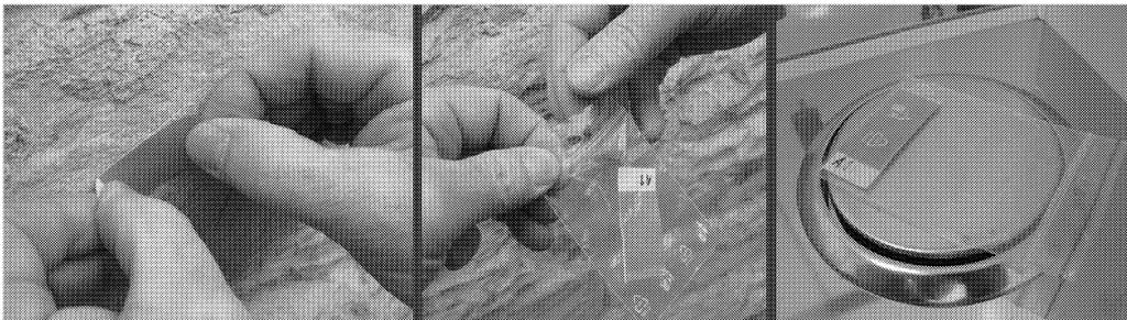
Fig.2: Basic steps of peeling test; a) strip being attached to the surface, b) saving removed material, c) weighing with laboratory scales
