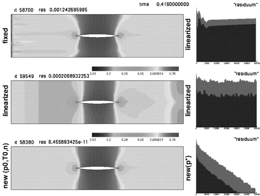
Fig.3: Incompressible flow, body in the channel; comparison of the various boundary conditions
