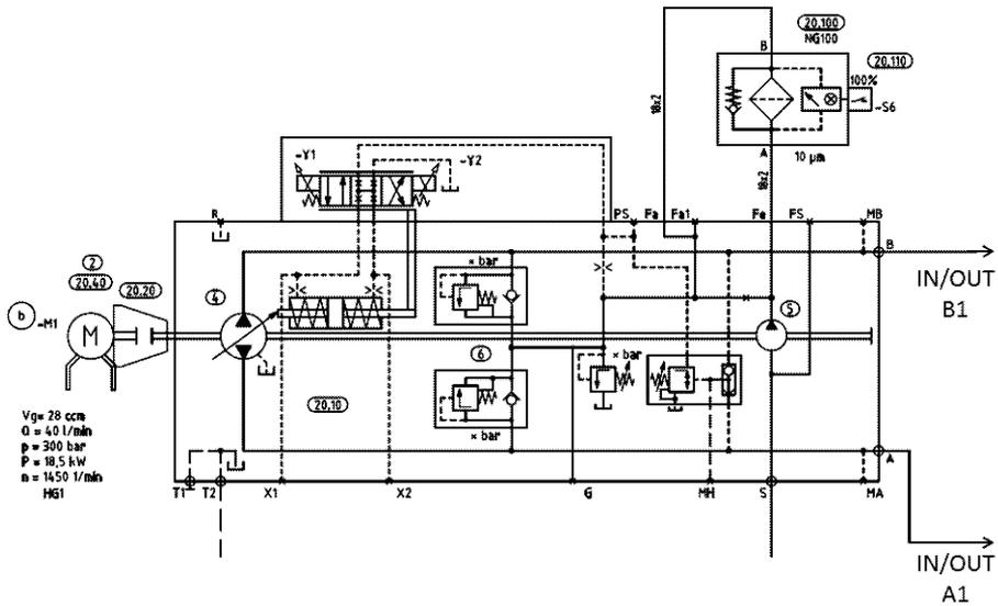
Fig.1a: The hydraulic scheme of the pump block
