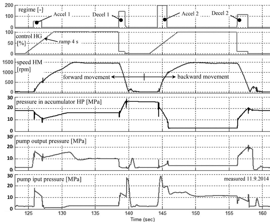
Fig.8: Measuring of cyclic run of the roller with energy recovery (roller mass: 18049 kg)
