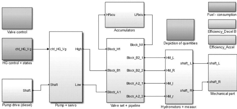
Fig.5: Embodiment of the pump subsystem into the whole model of the roller (3 shadowed blocks on the left hand side)
