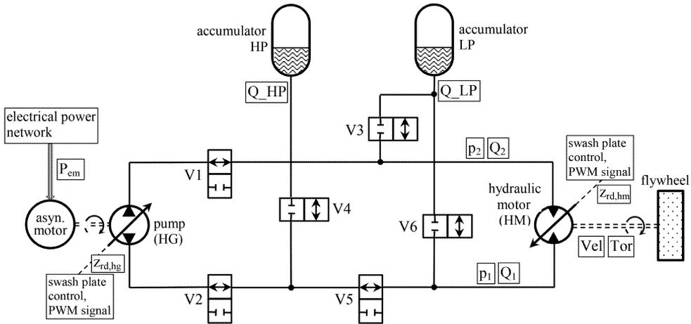
Fig.2: Simplified scheme of the PPHR with a controlled pump
