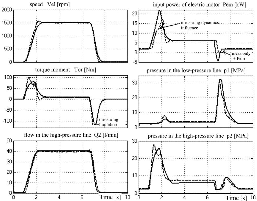
Fig.3: Simulated (full line) and measured quantities (dashed line) during acceleration and stop
