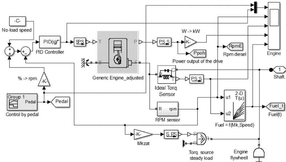
Fig.6: Model of diesel engine drive of the pump, including accessories and fuel consumption measurement
