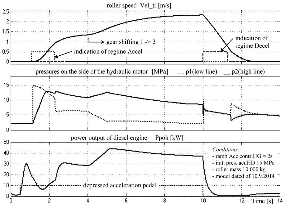
Fig.7: Start and stop of the roller, an example of simulated quantities courses
