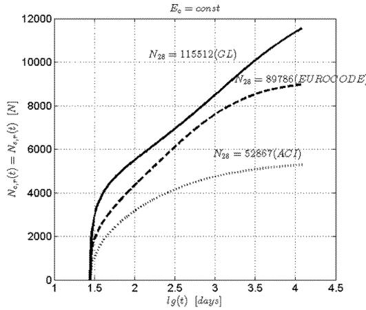
Fig.3: Normal forces  $N_{c,r}(t) = N_{a,r}(t)$ ,  $t = 12028$  days,  $t_0 = 28$  days, (humidity 80 %)
