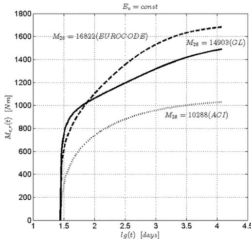
Fig.4: Bending moments  $M_{c,r}(t)$ ,  $t = 12028$  days,  $t_0 = 28$  days, (humidity 80 %)
