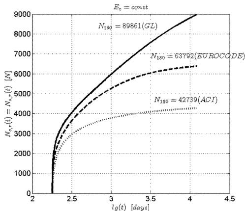
Fig.11: Normal forces  $N_{c,r}(t) = N_{a,r}(t)$ ,  $t = 12180$  days,  $t_0 = 180$  days, (humidity 80 %)
