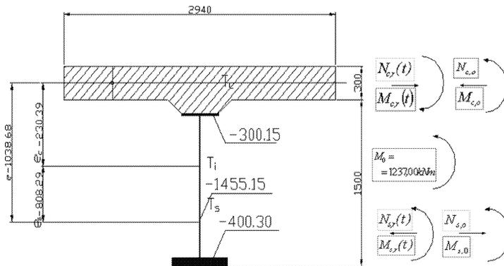
Fig.2: Composite beam with cross-section characteristic
