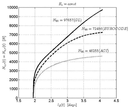
Fig.9: Normal forces  $N_{c,r}(t) = N_{a,r}(t)$ ,  $t = 12090$  days,  $t_0 = 90$  days, (humidity 80 %)
