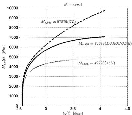
Fig.14: Bending moments  $M_{a,r}(t)$ ,  $t = 12365$  days,  $t_0 = 365$  days, (humidity 80 %)
