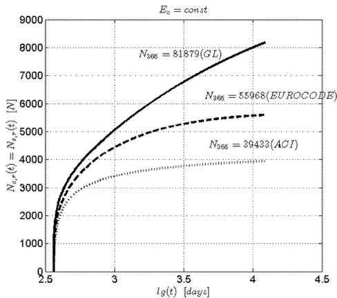
Fig.13: Normal forces  $N_{c,r}(t) = N_{a,r}(t)$ ,  $t = 12365$  days,  $t_0 = 365$  days, (humidity 80 %)
