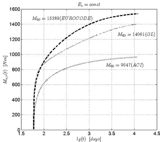
Fig.7: Bending moments  $M_{c,r}(t)$ ,  $t = 12060$  days,  $t_0 = 60$  days, (humidity 80 %)
