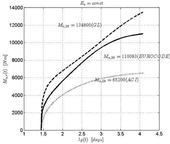
Fig.5: Bending moments  $M_{a,r}(t)$ ,  $t = 12028$  days,  $t_0 = 28$  days, (humidity 80 %)
