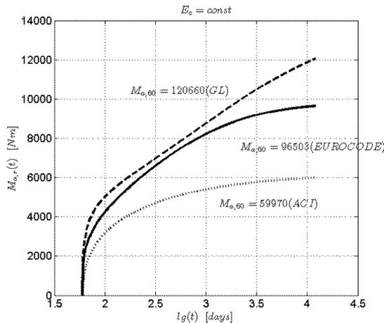
Fig.8: Bending moments  $M_{a,r}(t)$ ,  $t = 12060$  days,  $t_0 = 60$  days, (humidity 80 %)
