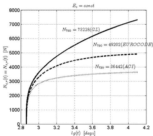
Fig.15: Normal forces  $N_{c,r}(t) = N_{a,r}(t)$ ,  $t = 12730$  days,  $t_0 = 730$  days, (humidity 80 %)
