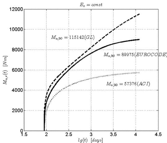
Fig.10: Bending moments  $M_{a,r}(t)$ ,  $t = 12090$  days,  $t_0 = 90$  days, (humidity 80 %)
