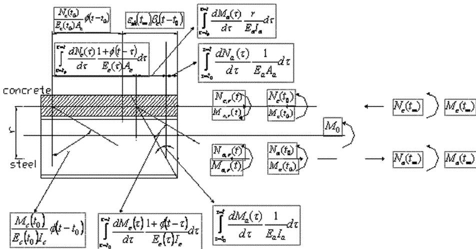
Fig.1: Mechanic-mathematical model for deformations in cross-section, regarding creep of the concrete
