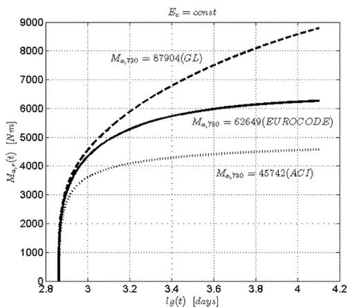
Fig.16: Bending moments  $M_{a,r}(t)$ ,  $t = 12730$  days,  $t_0 = 730$  days, (humidity 80 %)
