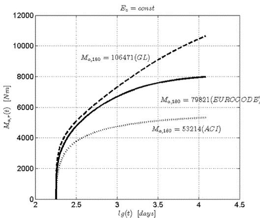
Fig.12: Bending moments  $M_{a,r}(t)$ ,  $t = 12180$  days,  $t_0 = 180$  days, (humidity 80 %)
