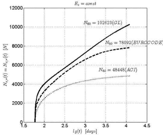
Fig.6: Normal forces  $N_{c,r}(t) = N_{a,r}(t)$ ,  $t = 12060$  days,  $t_0 = 60$  days, (humidity 80 %)
