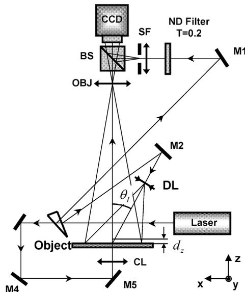
Fig.1: The optical set-up for out-of-plane measurement
