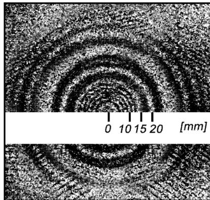
Fig.4: Subtraction fringe pattern representing propagation of the bending wave  $15 \mu\text{s}$  after impact
