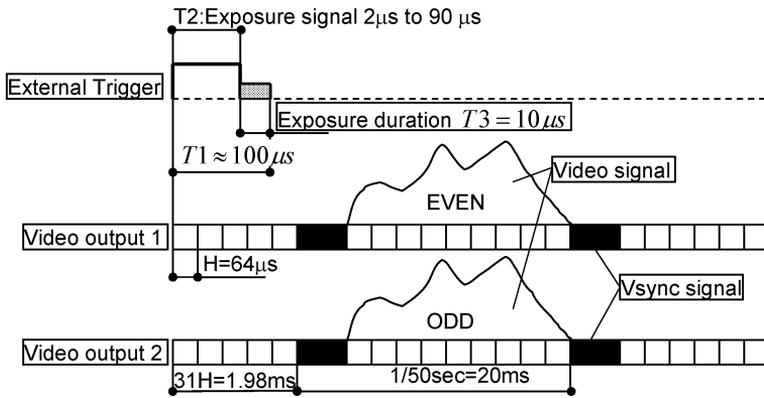
Fig.2: Timing chart for high-speed RESET mode video signal output
