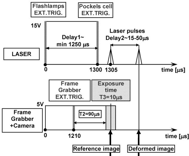
Fig.3: Pulse delay and pulse separation in electronic part of the interferometer
