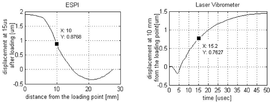
Fig.6: The comparison of ESPI and laser vibrometer results
