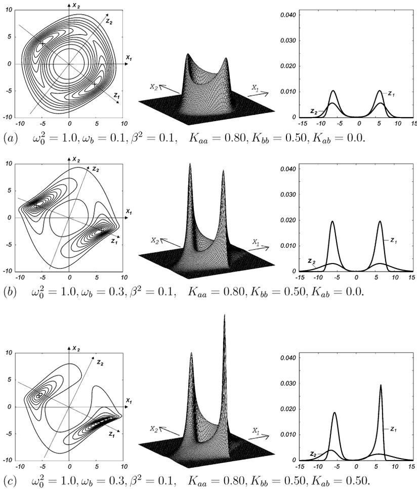
Fig.12: Van der Pol equation in the stationary state under simultaneous action of additive and multiplicative excitation; excitation processes  $w_a, w_b$ : independent ( $K_{ab} = 0$ ) – parts (a), (b) or correlated ( $K_{ab} > 0$ ) – part (c)
