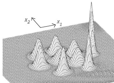
Fig.5: Axonometric display of the PDF evolution of an SDOF system response since the excitation beginning ( $t = 0$ ) until the stationary state ( $t = 90$  s)
