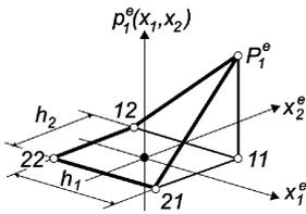
Fig.1: PDF approximation outline in a domain of one finite element
