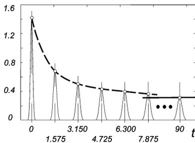
Fig.4: PDF vertical section  $x_1$  (deflection) in selected moments starting from the initial condition until the stationary state
