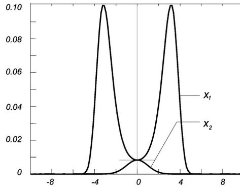
Fig.9: Vertical sections of PDF for Duffing system in the stationary state for  $K_{aa} = 0.2$ :  $x_1$ -deflection,  $x_2$ -velocity
