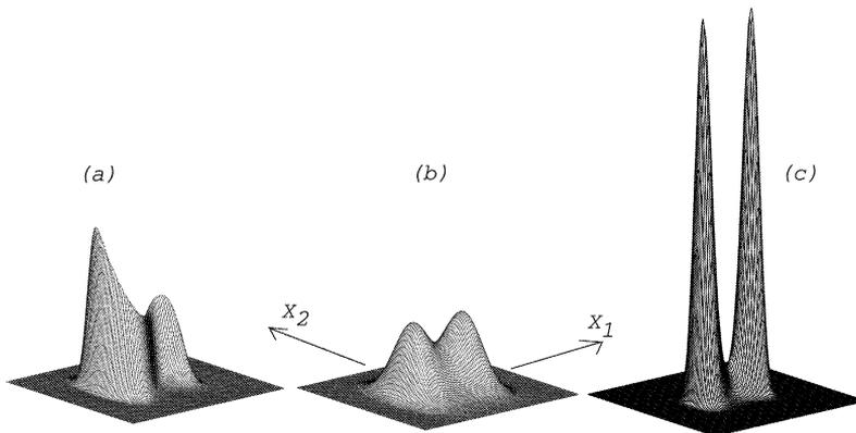
Fig.8: Axonometric display of PDF of the Duffing system response for  $K_{aa} = 4.0$  in the moment  $t = 4$  s and in the stationary state – parts (a), (b); stationary PDF for  $K_{aa} = 0.2$  – part (c)
