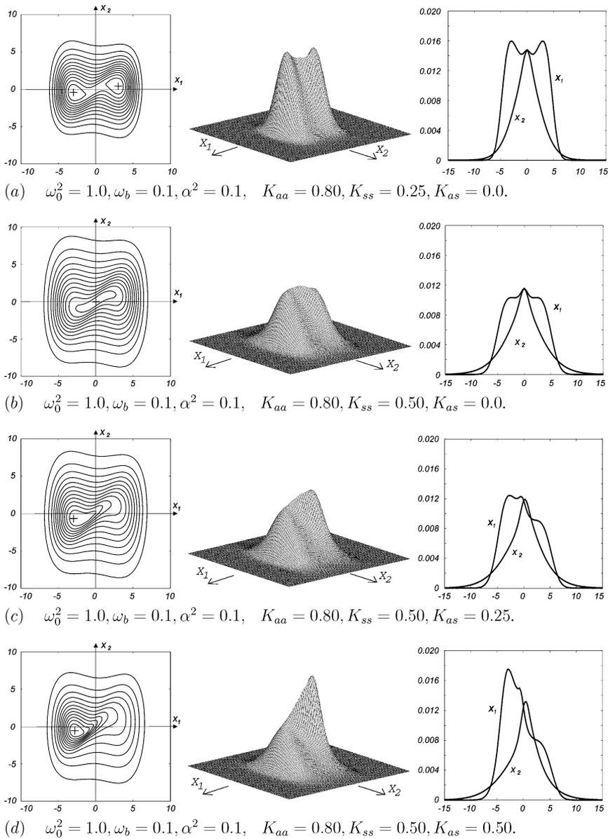
Fig.10: Duffing system in the stationary state under concurrent action of additive and multiplicative noises; excitation processes  $w_a, w_s$  are independent ( $K_{as} = 0$ ) – parts (a), (b); processes  $w_a, w_s$  are correlated ( $K_{as} > 0$ ) – parts (c), (d)
