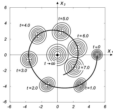
Fig.3: Contour diagram of the PDF evolution of an SDOF system response since the excitation beginning until the stationary state
