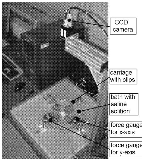
Fig.1: General view of the testing rig
