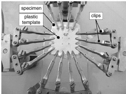
*Fig.2: Clamping of specimen using a plastic template*
