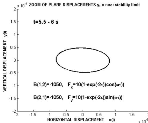
Fig.13: Apparent stable plane trajectory at  $B(1,2) = B(2,1) = -1050$
