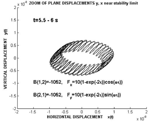
Fig.10: Plane trajectory at  $B(1,2) = B(2,1) = -1052$
