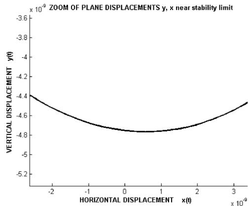
Fig.15: Plane trajectory without high frequency component at  $B(1,2) = B(2,1) = -1049$
