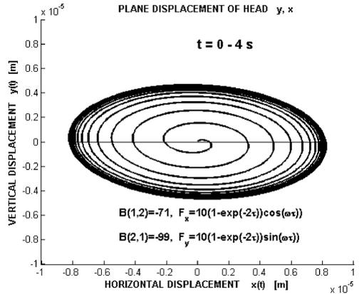
Fig.2: Plane trajectory of bearing head motion
