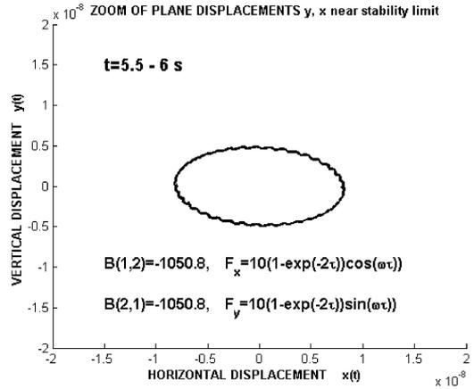
Fig.12: Plane trajectory with small higher frequency component
