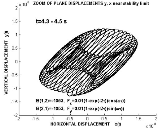
Fig.8: Plane trajectory of unstable motion for  $t = 4.3-4.5$  s
