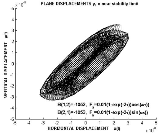
Fig.6: Plane trajectory of unstable motion at  $B(1,2) = B(2,1) = -1052$
