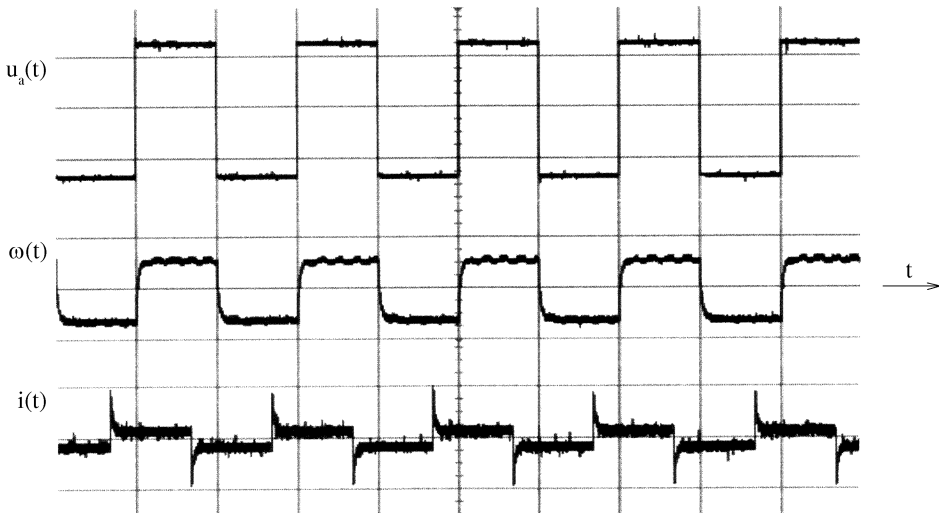
Fig.7: Time signal of feeding voltage u_a(t) , induced voltage u_i(t) and armature current i(t) , one period
