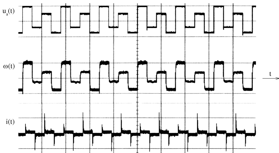
Fig.8: Time signal of feeding voltage u_a(t) , induced voltage u_i(t) and armature current i(t) , two periods
