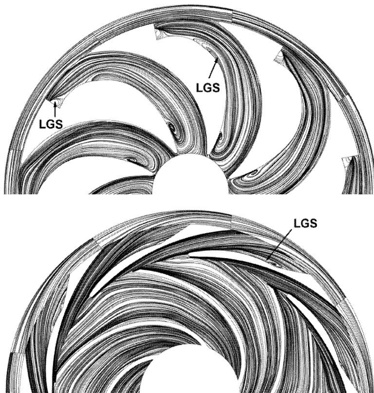
Fig.10: Streamlines on Plane1 and Plane2; pump mode,  $Q = 11.4\text{ l/s}$ ;
