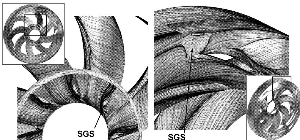
Fig.7: Separations in the stator; turbine mode, full impeller,  $Q = 15.75$  l/s; SGS means a small global separation
