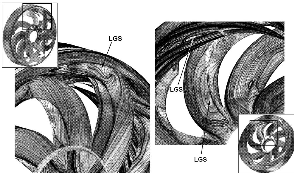
Fig.11: Separations in the stator; pump mode,  $Q = 11.4\text{ l/s}$ ;
