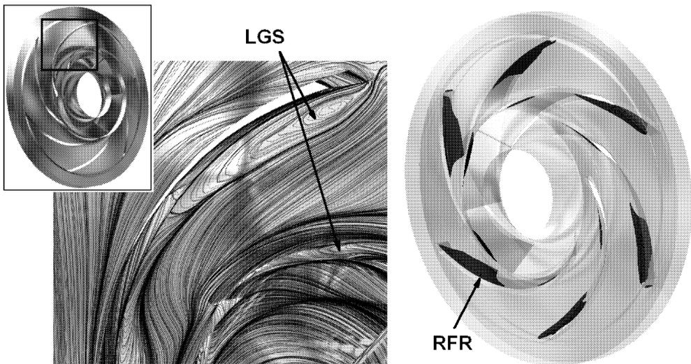
Fig.9: Global separations in the rotor and the visualization of the reverse flow regions in the rotor passages; turbine mode, reduced impeller,  $Q = 13.5 \text{ l/s}$ ; LGS means a large global separation, RFR means a reverse flow region
