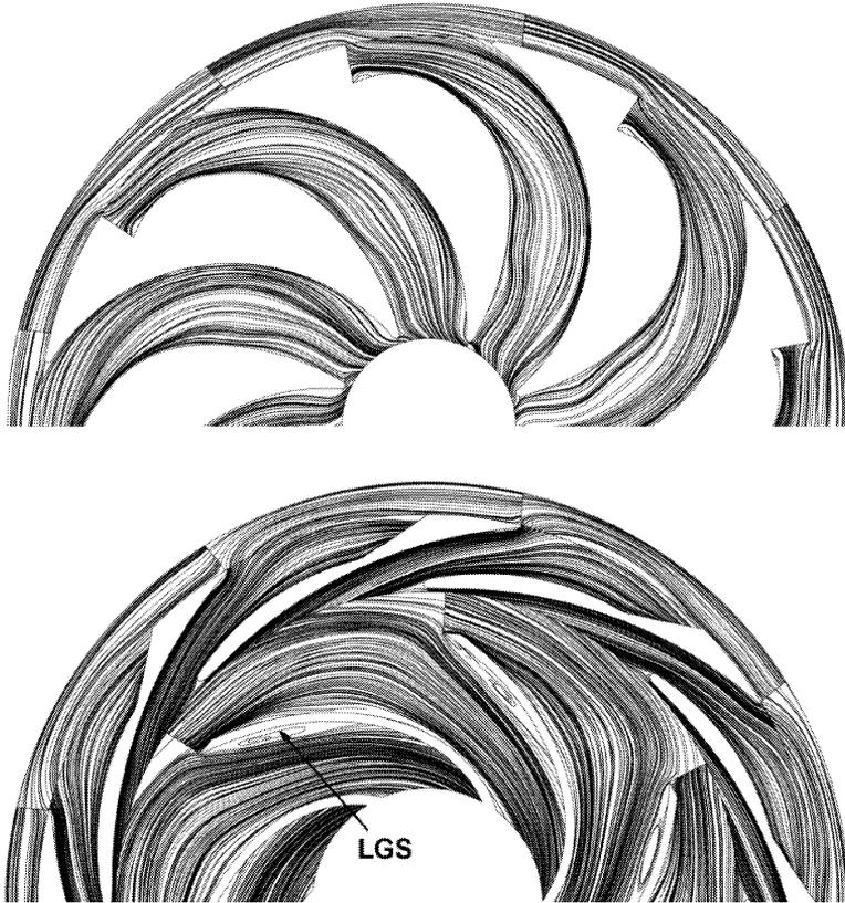
Fig.8: Streamlines on Plane1 and Plane2; turbine mode, reduced impeller,  $Q = 13.5 \text{ l/s}$ ; LGS means a large global separation
