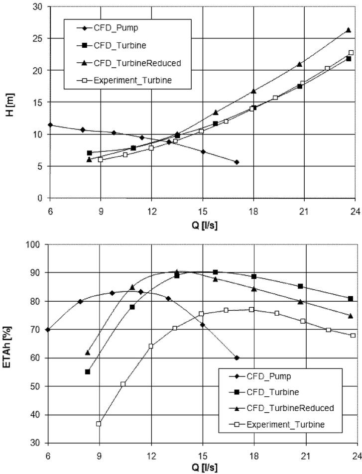
Fig.4: Calculated head and hydraulic efficiency in the pump and turbine regimes and measured head and overall efficiency in the turbine regime
