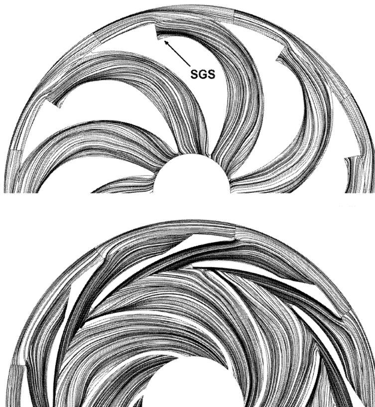
Fig.6: Streamlines on Plane1 and Plane2; turbine mode, full impeller,  $Q = 15.75$  l/s; SGS means a small global separation
