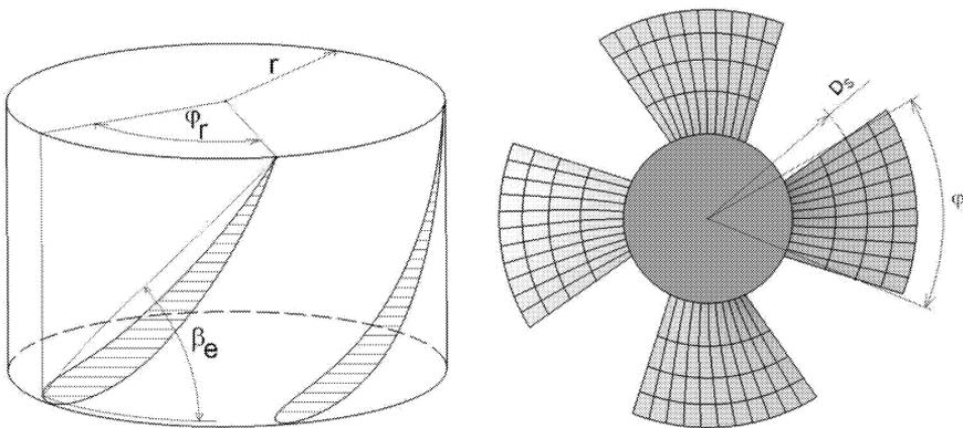
Fig.5: View on the cylindrical blade sections
