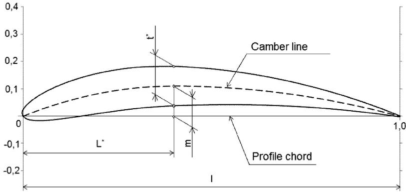
Fig.9: Main dimensions of NACA airfoil
