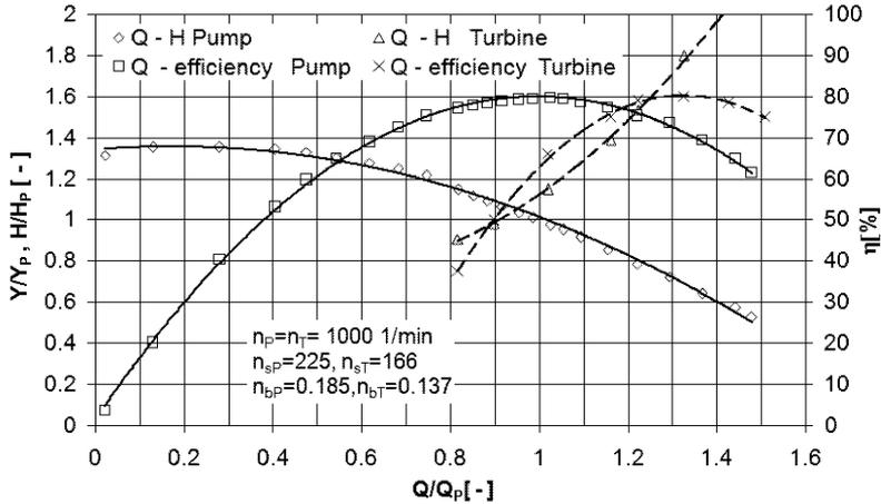
Fig.2: Characteristic of the pump and the turbine
