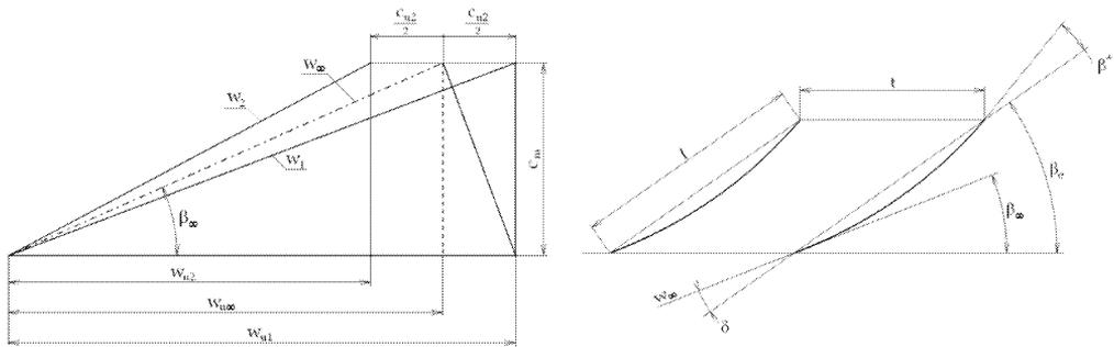
Fig.4: Velocity triangles and the cascade of axial pump
