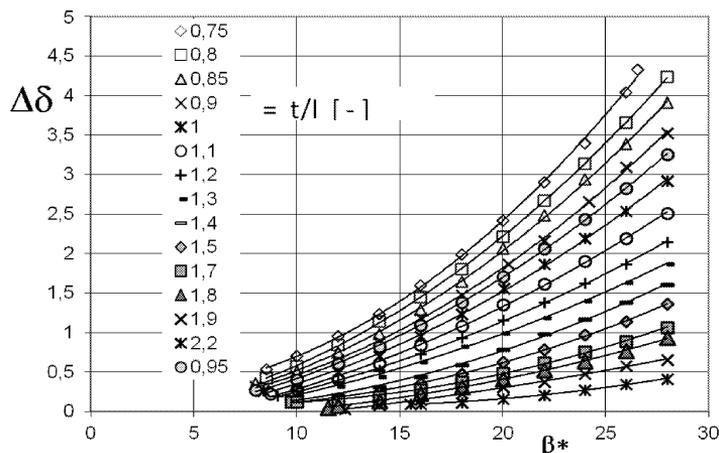
Fig.8: Dependency of a difference of an angle of attack  $\Delta\delta$  on relative pitch  $t/l$  and angle of an airfoil deflection  $\beta^*$  of a blade cascade  $\beta_e$
