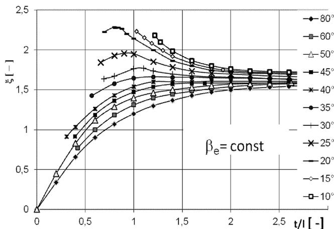
Fig.7: Dependency of a coefficient of cascade's impact  $\xi$  on relative pitch  $t/l$  and angle of a blade cascade inclination  $\beta_e$
