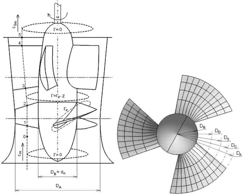
Fig.1: The main dimensions of the axial turbomachine
