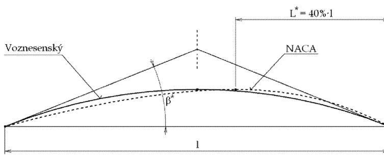
Fig.6: Centerline of the NACA profile compared to an equivalent circular arc of Voznesensky
