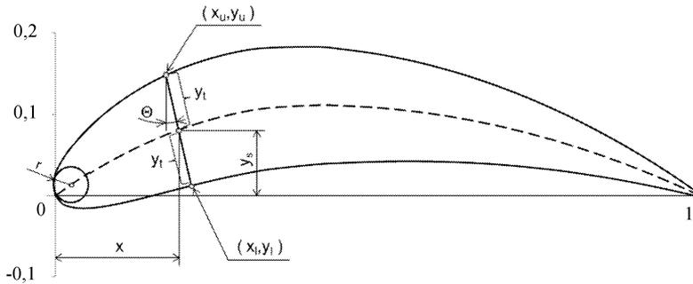
Fig.10: NACA airfoil – determining of vertices
